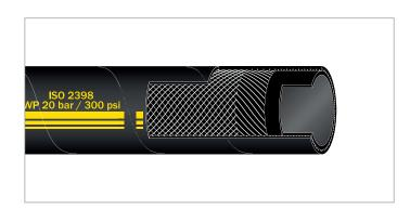
Code - A8G01.... Base Material - SBR Operating Temperature - -30 ÷ +70 °C Pressure - 20 bar Vacuum - n.d. Diameter Range - 6 ÷ 32 mm Key Feature - Reinforced
